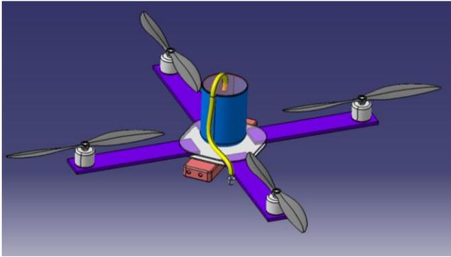
Fig. 1. Assembly of quad copter with spraying mechanism
