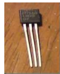
Figure 4: LM35 pin number and TO-92 Plastic Package.
