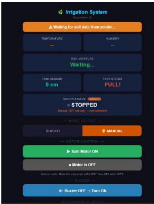
FIGURE 5 : WEB TERMINAL OF IRRIGATION SYSTEM (MANUAL PUMPING)
