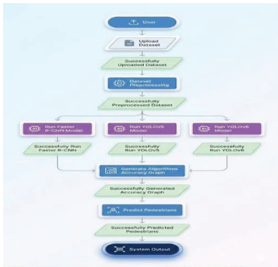
Fig. 2. System workflow for pedestrian detection.
