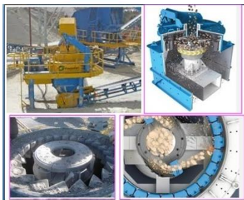
Fig.1 Vertical Shaft Impactor (VSI) for producing M-Sand
