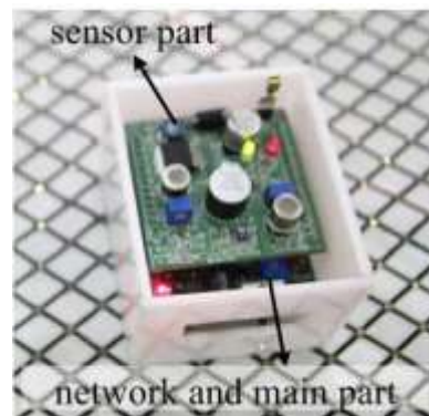
Fig. 2. Prototype of the ZiSAS.
