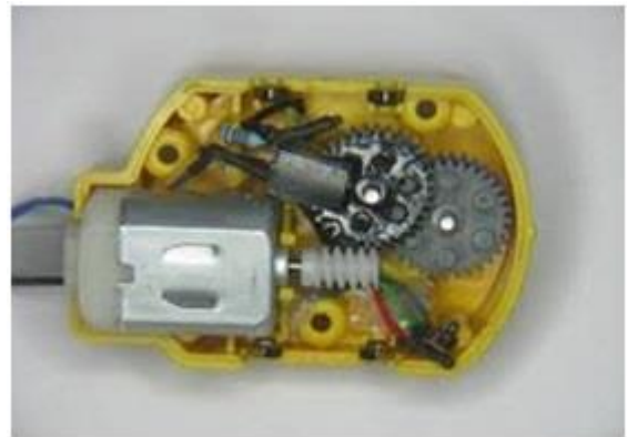
Fig.3 DC motor and gear structure used in the joint of the robot
