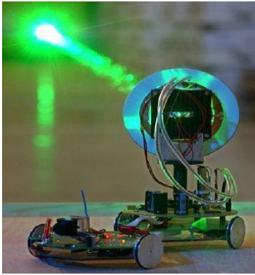
Fig.6 EADS developed fully laser power autonomous rove
