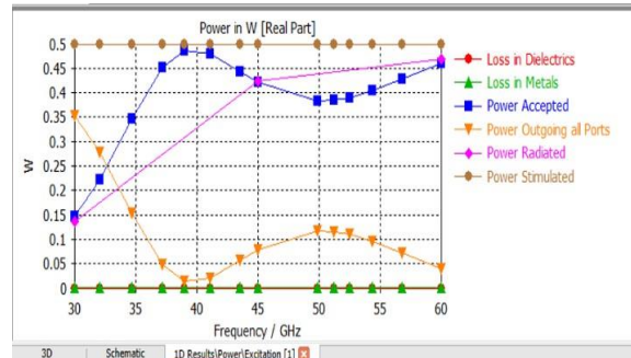
Fig. 7 Simulated power 0.5W, power accepted at all port by the antennas is 0.4832W.
