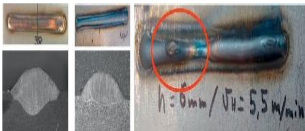
Fig.-5: Beads obtained by Top-TIG on AISI 316L. Left) 1 kg/h. Centre) 1.5kg/h. Right) 1.6 kg/h.
