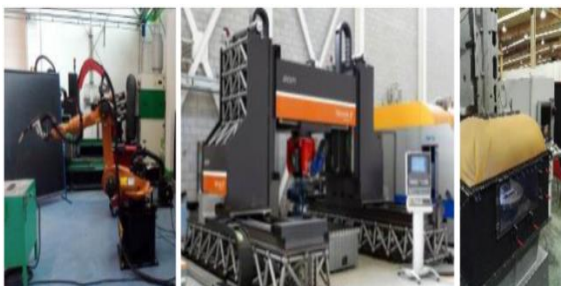
Fig -1: WAAM Facilities. Left- IK-4 Lortek (CMT & TopTIG). Centre-TECNALIA (PAW). Right- ADDILAN (CMT&PAW)
