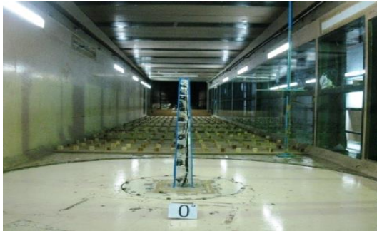
Fig. 4. Typical view of the model oriented at \theta = 0^\circ in wind tunnel
