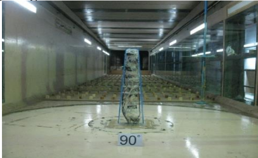
Fig. 5. Typical view of the model oriented at \theta = 90^\circ in wind tunnel
