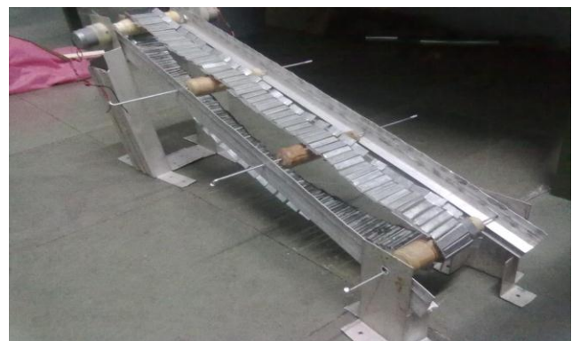
Fig.2 Setup of the Coal Drying System
