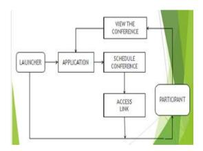
From the dataflow diagram, the launcher with the help of application can schedule the conference once the launcher schedule the conference it process an access link. Using this access link the participant can view the conference.
