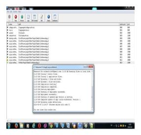
Once the user application is successfully created in the app engine, then the user can launch his application in the Google App engine Launcher. To launch a application add an existing application from the file, click on run and wait for green mark at the beginning of the application name, latter click on browse. By this way user can launch the application in the Google app engine Launcher.
