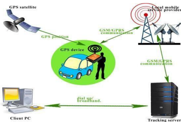
Fig. 1. Architecture of the vehicle tracking, monitoring, and security system.
