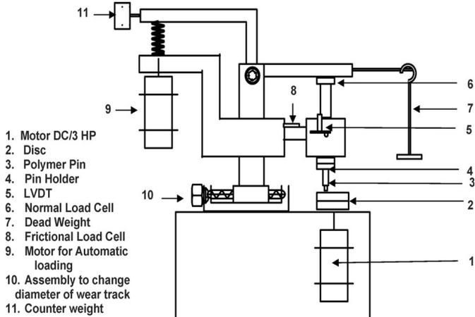
Fig. 2. Schematic showing the pin on disc machine.
