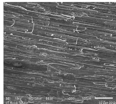
Fig. 5. Scanning electron micrographs of worn surface speed 1m/s & load 150 N
