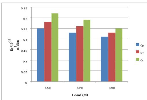
Fig. 3. Friction coefficient under various loads for composites in adhesive wear
