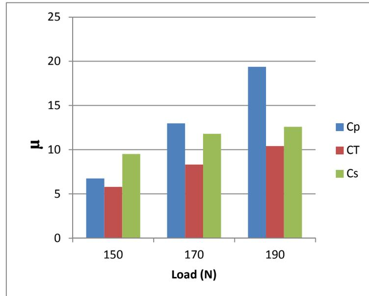
Fig. 4. Specific wear rate ( $K_o$ ) under various loads for selected composites in adhesive wear mode
