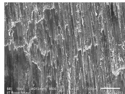
Fig. 6. Scanning electron micrographs of worn surface speed 1m/s & load 170 N
