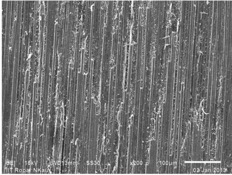
Fig. 7. Scanning electron micrographs of worn surface speed 1m/s & load 170 N
