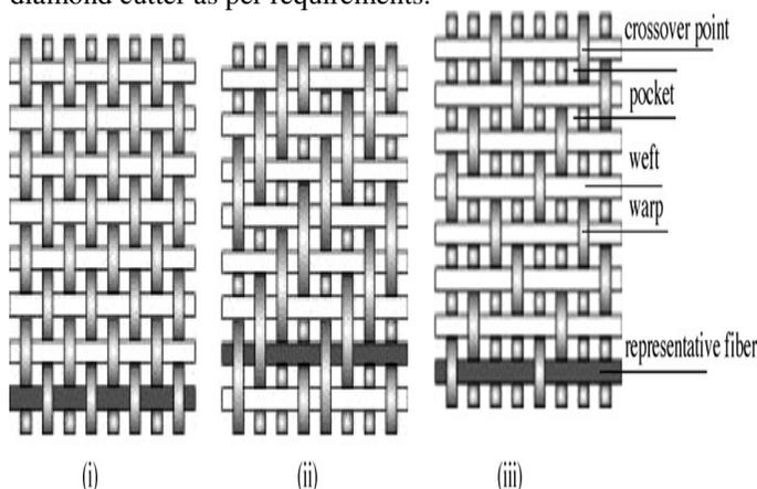
Fig.1. Schematic showing different weave patterns: (i) plain, (ii) twill and (iii) satin (4-H)
