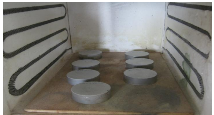
Fig. 2.1 Pellets Formed From Elemental Powders
