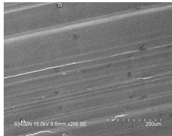
Fig 12: SEM morphology of worn surface of spray-deposited and hot pressed alloy at the load of 68.67 N.
