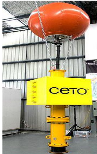
Fig.4. CETO Float and Pump Unit prior to deployment
