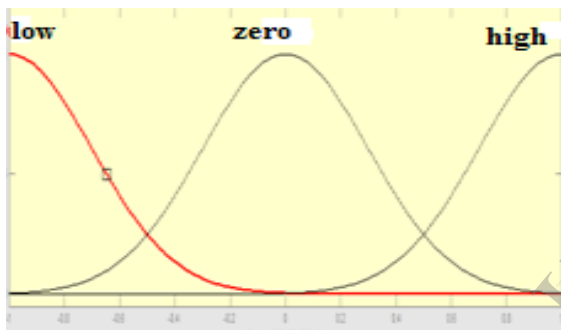
Fig.6.Membership function characterizing the input variable 'deviation'
