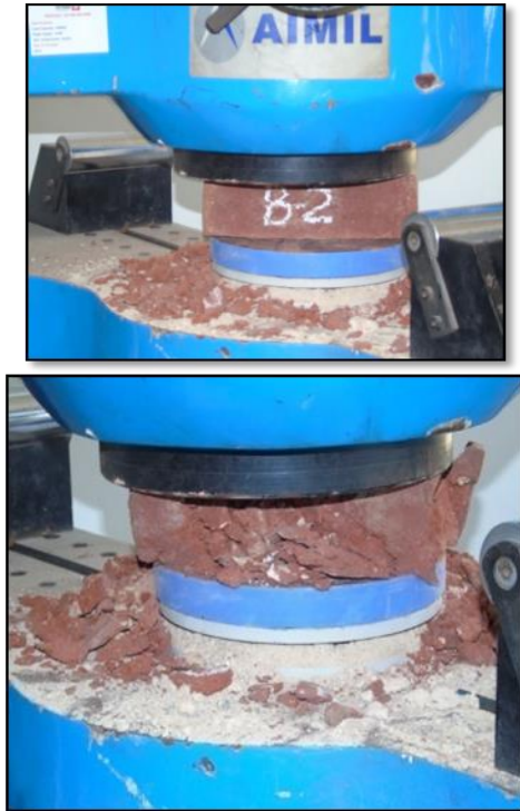
Figure-3.5a: Compression Test on UTM
