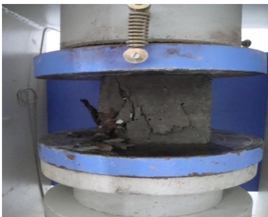
Fig. 3 Set up for compressive strength test in compression testing machine.
