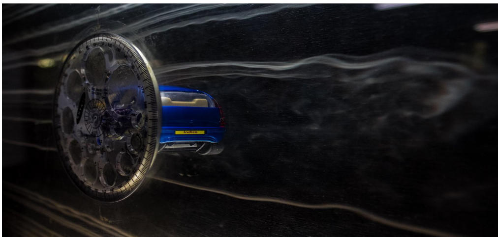
Figure 11(b) Wake visualization behind the car
