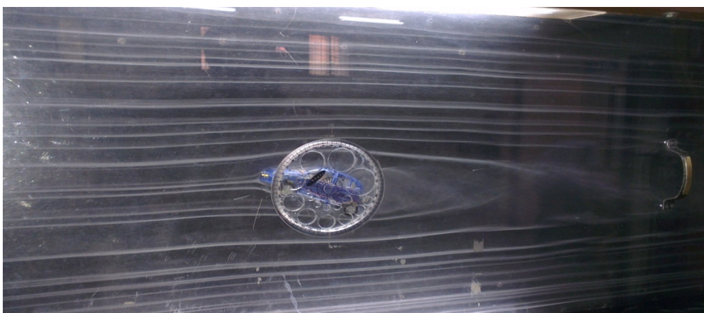
Figure 11(c) Wake visualization at positive 15 degree angle.
