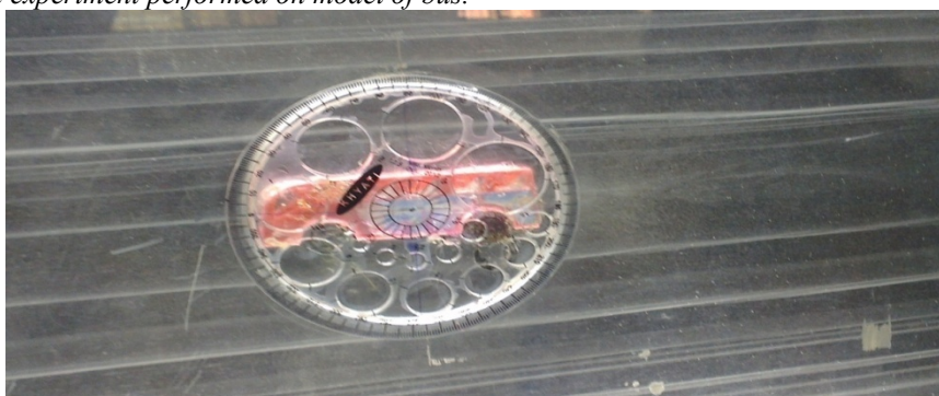
Figure 14(a) Flow visualization of Bus model in test section
