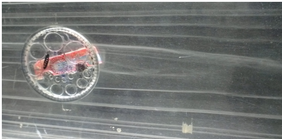
Figure 14(e) Flow visualization behind the Bus model at negative 10 degree angle
