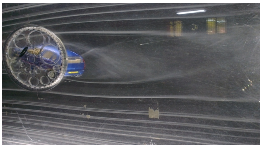
Figure 11(d) Wake visualization behind the car at positive 15 degree angle.
