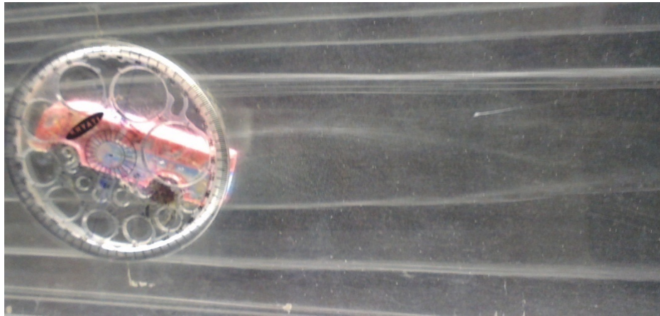
Figure 14(d) Flow visualization behind the Bus model at positive 15 degree angle
