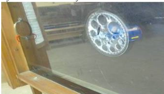
Figure 8(a) Hatchback model fitted in test section of Smoke Tunnel Figure 8(b) Wooden model of sedan fitted in test section
