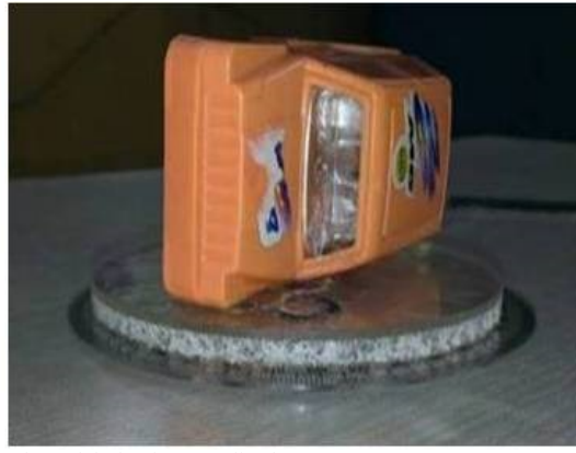
Figure 5(a) Hatchback model glued on acrylic sheet Figure 5(b) Squareback model is glued on acrylic sheet
