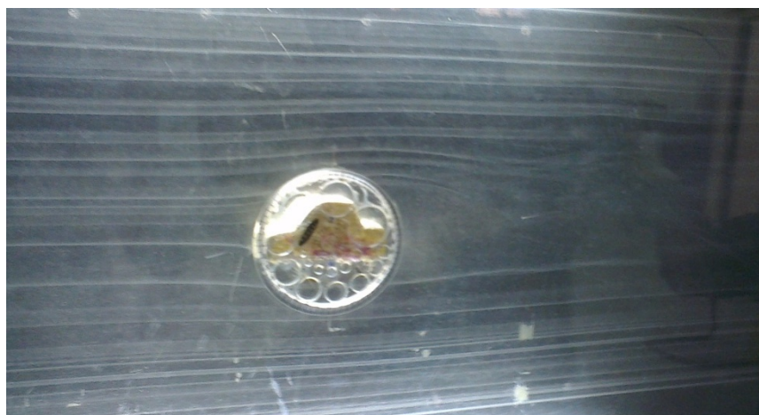
Figure 12(b) Wake visualization behind the sedan model
