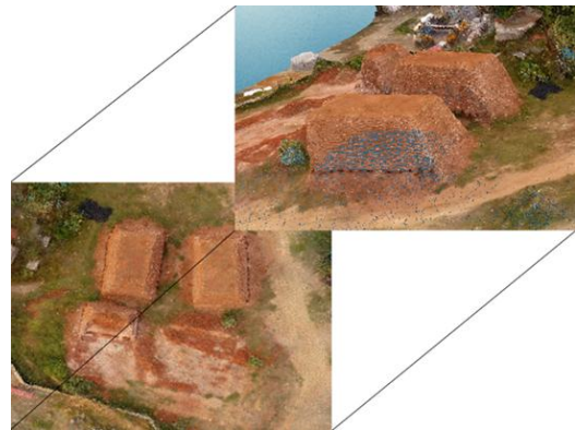
Figure 6: SFM Generated Point Cloud
