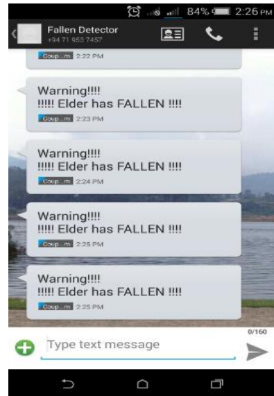
Fig. 17: SMS sent to the caretakers about the fall
