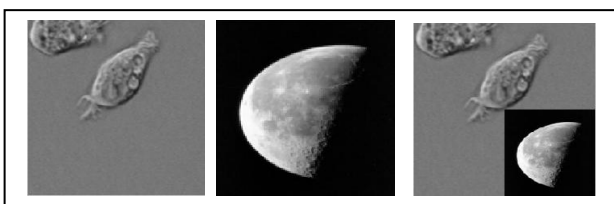
Fig. 2.DCT method_Test2: (a) Original image (b) watermark image (c) watermarked image
