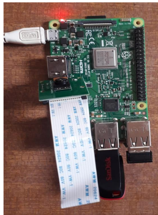
Fig.1 RaspberryPi connection with different component Fig 1. shows raspberry Pi connected with different components such as power source, mouse , pendrive and raspberry pi camera.
