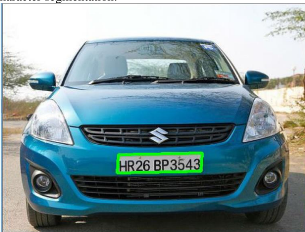
Fig.4. Vehicle registration number plate detection
