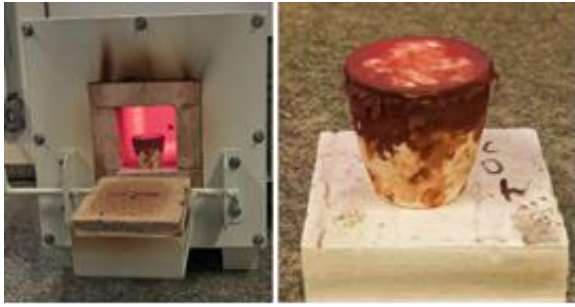
Figure 3. After cementation, the crucible is removed from the muffle furnace to cool slowly.
