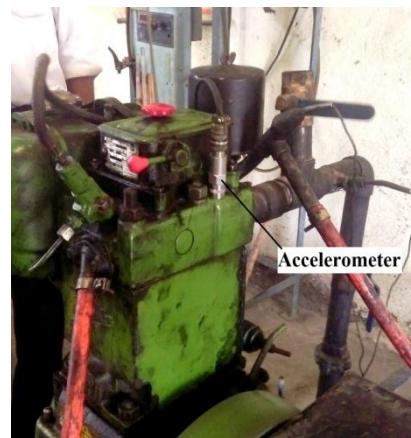
Fig. 3.2 Accelerometer mounted on Cylinder Head
