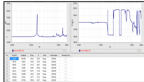
Fig. 23. Experimental results for surface crack at 80° for CCFF boundary conditions
