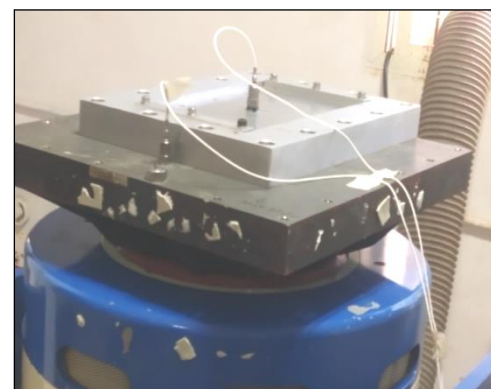
Fig. 7. Vibration shaker with plates for CCF boundary condition
