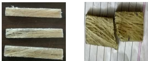
Fig. 4. Test Specimen before test and after impact test
