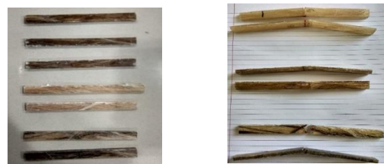
Fig. 3. Test specimen before test and after flexural test
