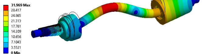
Fig.No.11 Total deformation of mode 6original Driveshaft
