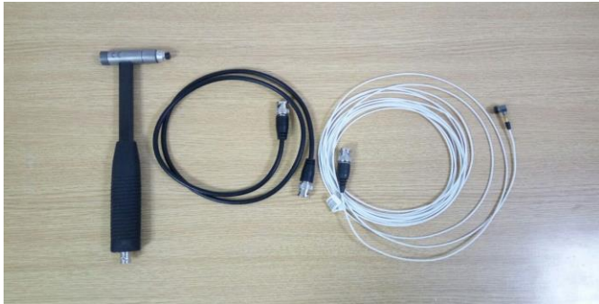
Fig. 4 Impact Hammer and P20 sensor
