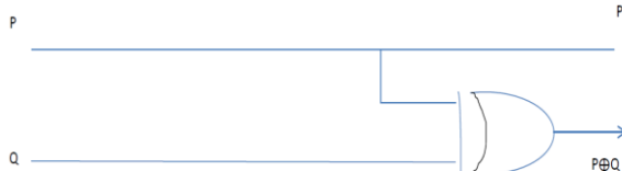
Fig 6 Combinational circuit of FEYNMAN gate
