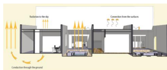
Fig. 5: Thermal performance analysis of courtyard at night(source:Haeri, 2010b).
