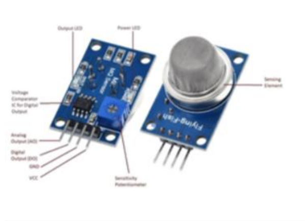
Fig(b): Sensors (Smoke & Vibration)
