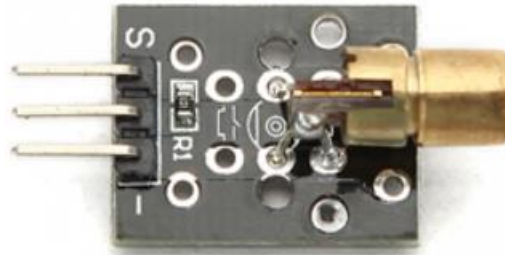
Fig(c): Li-Fi Transmitter
