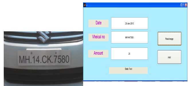
Fig. 12.1. Number plate and its recognized characters are shown in GUI
