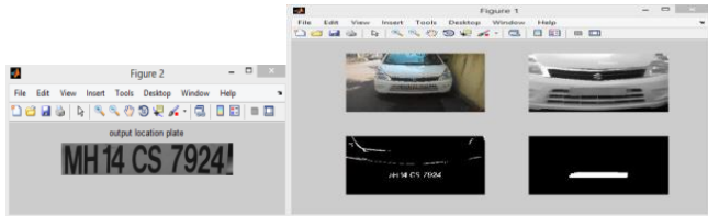
Fig. 6. Number Plate Extraction and Captured Number Plate
