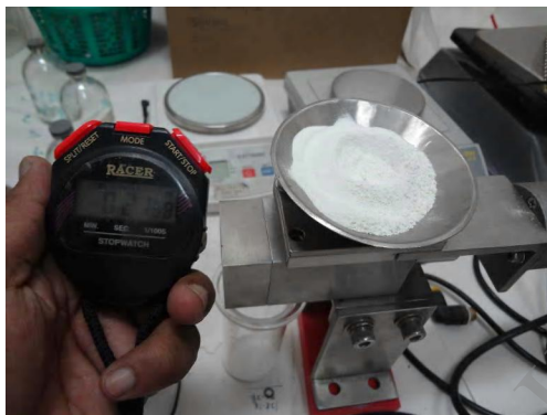
Fig. 10. Timer used for measuring the time taken by the dispenser to deliver the powder
