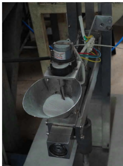
Fig.13. VDCSFPD with stirrer in operation during experiment with inactive Zr-Mo powder
