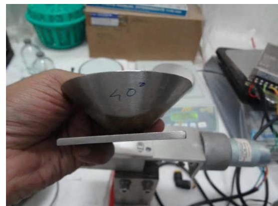
Fig. 8. SS conical hopper having \phi_s = 40^\circ ready for assembling with the dispenser
