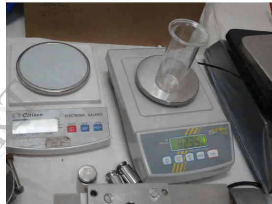
Fig. 6 Electronic balance for measuring the mass of the powder and volumetric beaker
