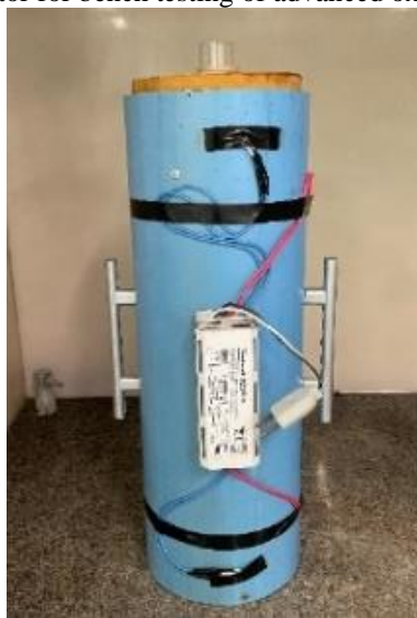
Figure 1 – Reactor for bench testing of advanced oxidation processes
