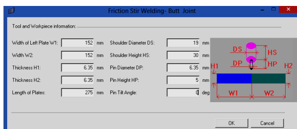
Fig.4 Tool & workpiece information input in HyperWeld.
