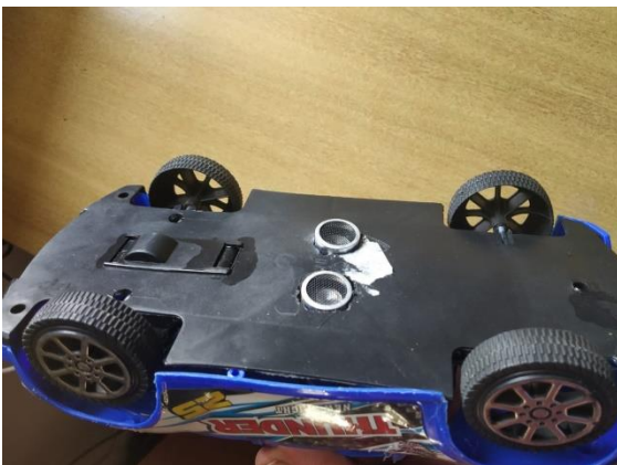
Fig 5. Ultrasonic sensor attached to the bottom of the car chassis to detect the potholes and humps.
