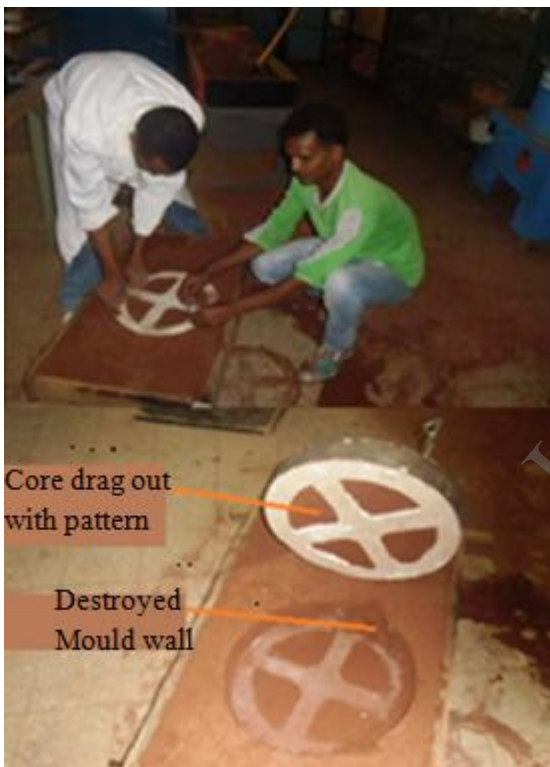
Fig. 3. Photograph indicating destroyed mold while removing a pattern.
