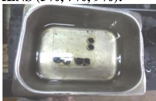
SPECIMENS OF SOFTENING POINT
