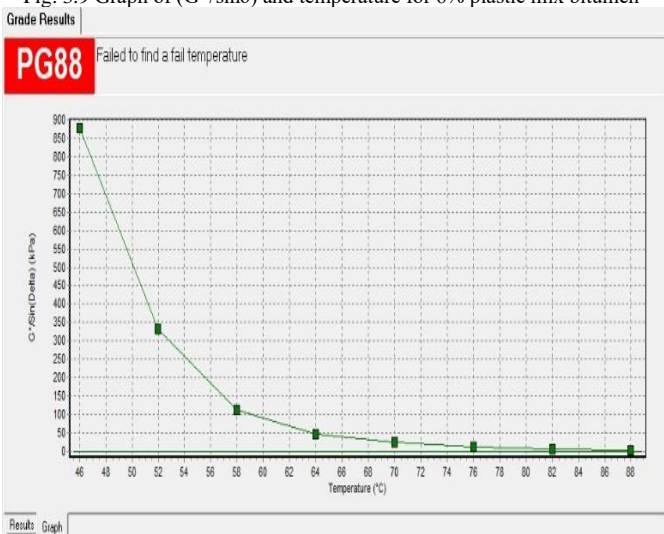
Fig.3.10 Graph of ( G^*/\sin\delta ) and temperature for 8% plastic mix bitumen
