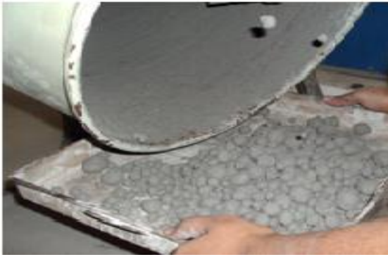
Figure: 1 showing process of formation of fly ash aggregates by pelletization.
