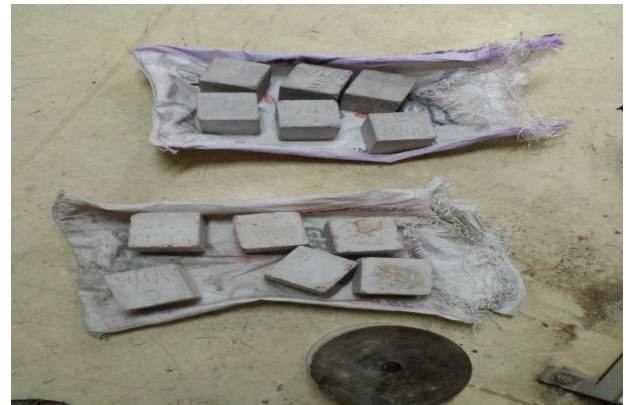
Fig. 7 cubes taken out of Na 2 SO 4 and H 2 SO 4 solution after first week
