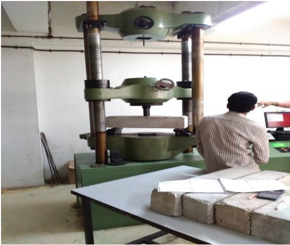
Fig. 2 Setup for centre point loading for flexure testing
