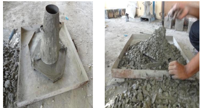
Fig 3: Slump cone and collapse of concrete after lifting
