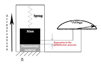
An electromechanical transducer is capable of converting mechanical vibrations into electrical voltages. Depending upon their sensing element and output characteristics, such pickups are referred to as accelerometers, velocity pickups, or displacement pickups. When the vehicle moves over bumps on the road these vibration pickups come into play and generate electricity which complements the accelerometers and improves the overall efficiency of the hybrid system.
