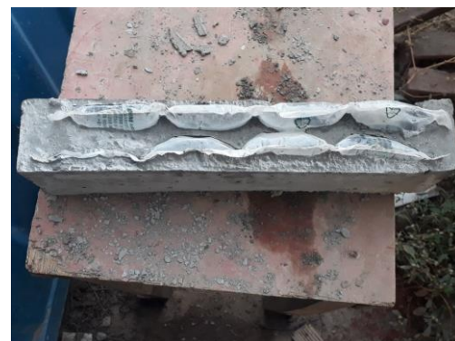
Figure 10 concrete block with insulating air bubble pouches inside
