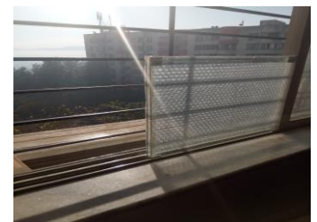
Figure 7 sandwich glass with air bubble sheet
