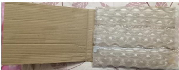
Figure 9 air wavy strips sandwiched in card board
