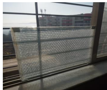
Figure 8 single glass with a backing of air bubble sheet
