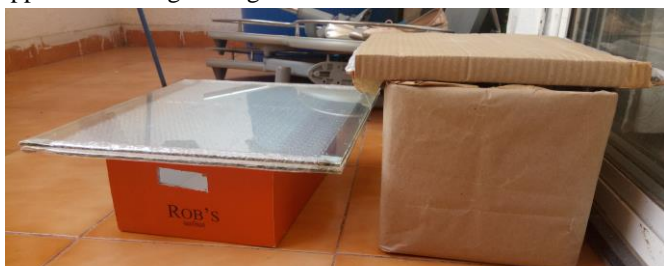
Figure 9: comparison between two covering panels, glass & cardboard sequentially.
