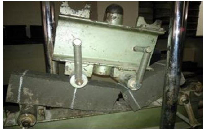
Fig -4: failure of flexure specimen
